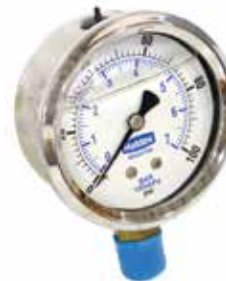
Port: 1/4 in.; Silicone Filled 0-100 PSI
